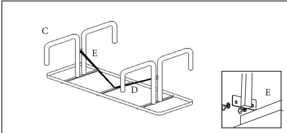
3. Connect table brace (D) to the table support (C) with bolts (E) loosely.
