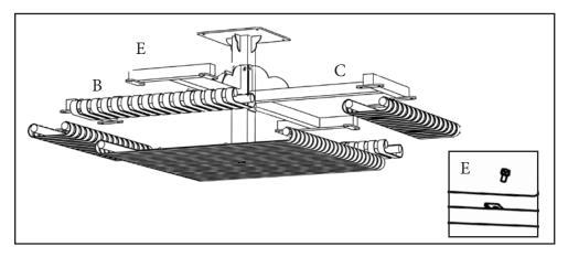
4. Connect seats (B) with seat supports(C), and insert bolts(E) loosely.
