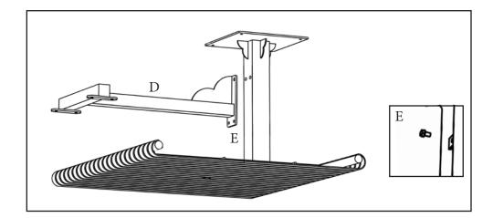
3. Connect seat supports (D) to the middle of table support (C) with bolts(E) loosely.
