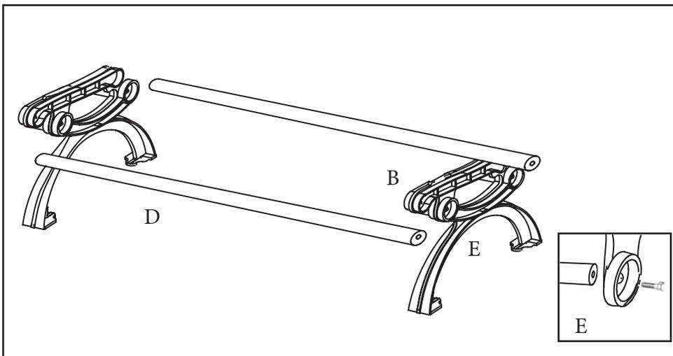
1. Assemble the supporting rods (D) and the seat supports (B) with four larger bolts and washers (E). Insert bolts (E) loosely.
