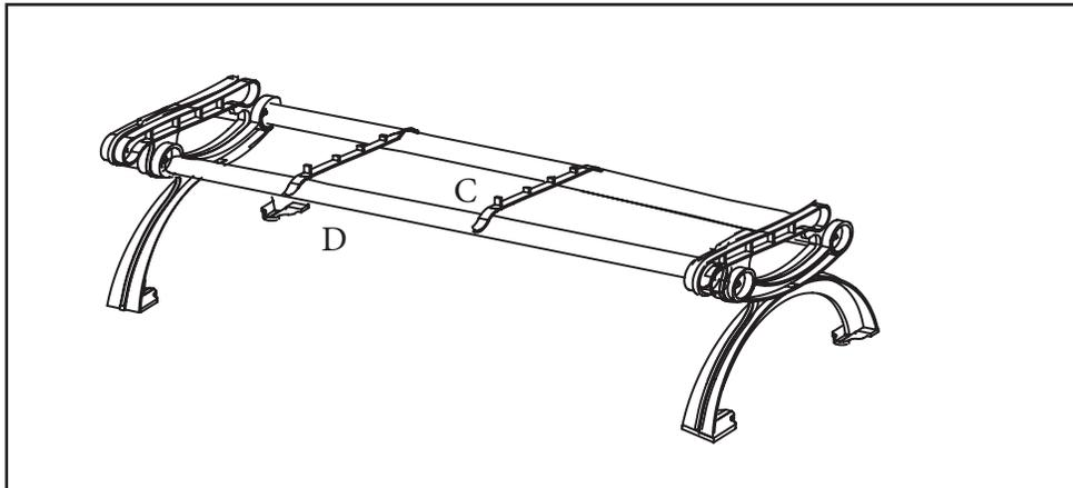
2. Equally space the two seat/backrest supporting brackets (C) onto the supporting rods (D).
