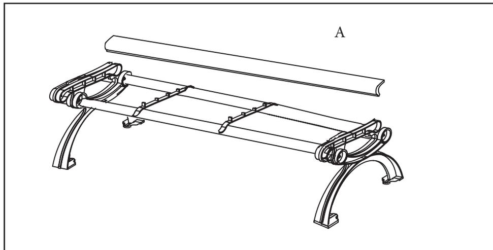
3. Sliding recycled plastic slabs into place. Seating has five slabs backrest has four slabs. Use the waterfall-edge recycled plastic slabs for the edges (A) and straight-edge slabs (B) between C.
